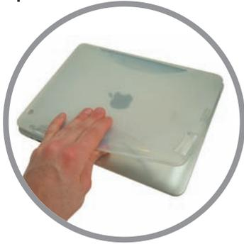
If using the iPad 2 or iPad 3 please insert the iPad into the silicon protective sleeve provided, to minimise movement within the enclosure.
