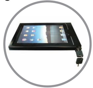
Slide cover back into position and secure with lock.
